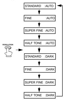
**Note:** In order to transmit in FINE or SUPER FINE resolution, the receiving fax machine must also have that resolution. If it doesn't, your machine will automatically step down to the next best available setting.
